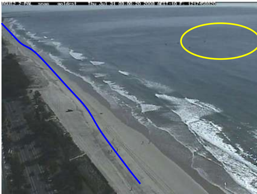
Figure 6: Narrowneck Beach showing the wider beach on the south side of the reef including a new depositional sand dune immediately south of the reef. Notably, offshore of the reef, many fishing boats are using the reef as a source for their catches. The blue line shows the high tide line.
